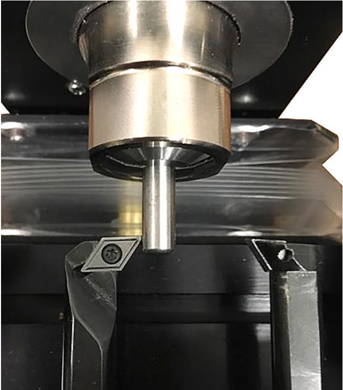
FIGURE 11—Notice the carbide tip on the left just touching the side of the dowel
