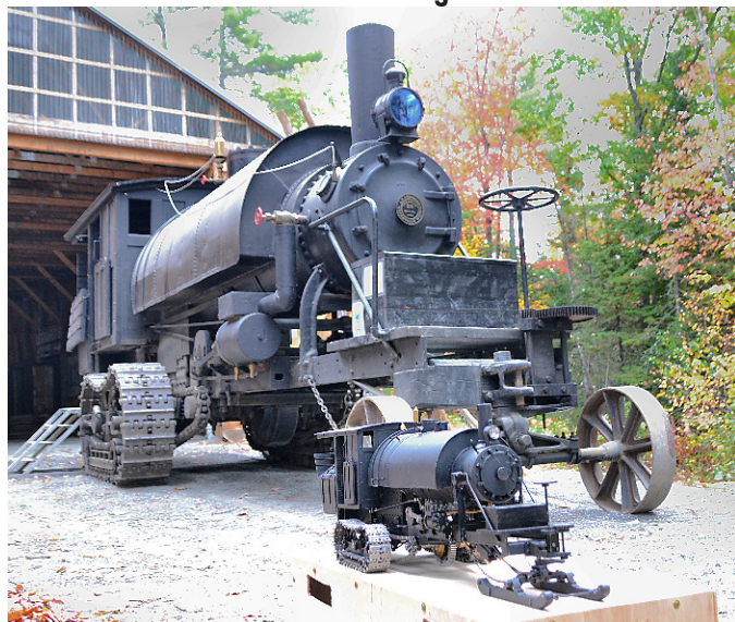
FIGURE 1—A Lombard log hauler completed last year, also done completely on his Sherline machines. Here is a shot of the model with its big brother at the Maine Forest and Logging Museum last fall, where both were running together.
