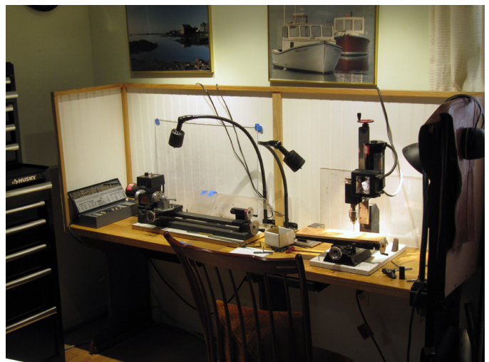
FIGURE 10—Chris's home-shop setup. The lathe is a 4400 model with a 17" base, and the mill is a 5400 model with a 12" base and an optional extended, 15" Z-axis column bed.
