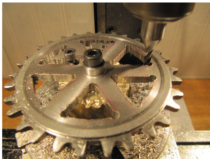
FIGURE 3—Machining a track wheel for the Lombard.
