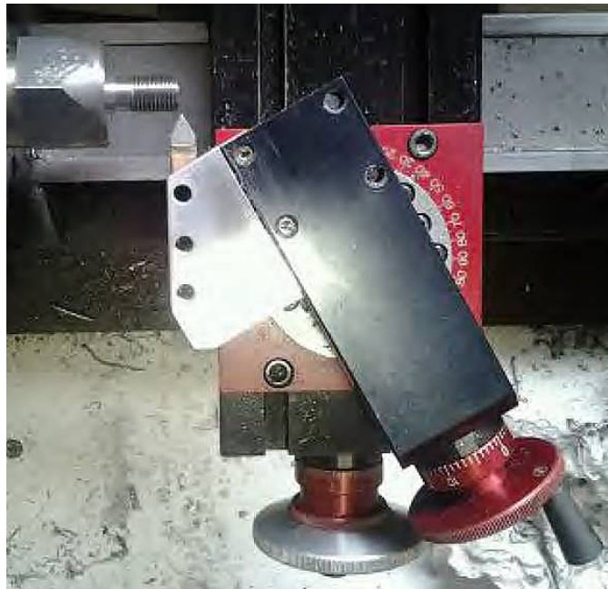
FIGURE 1—James’ custom tool holder mounted to the compound slide and cutting threads.
