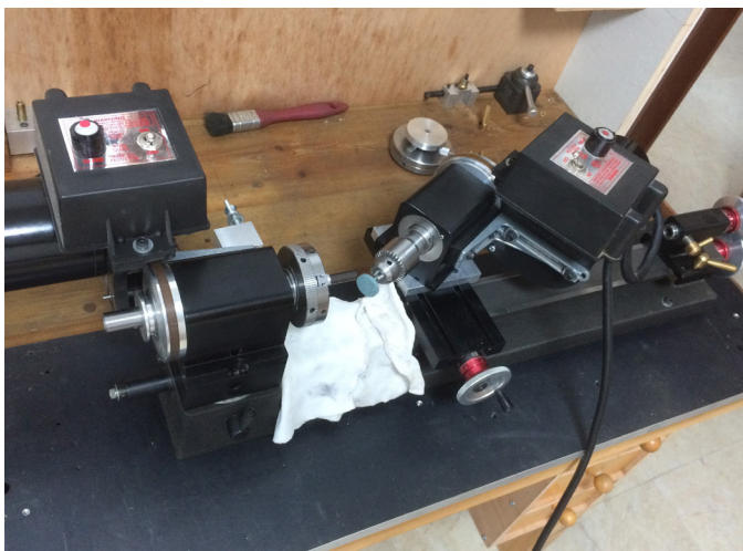
PICTURE 11—Another view of the angled crossslide headstock.
