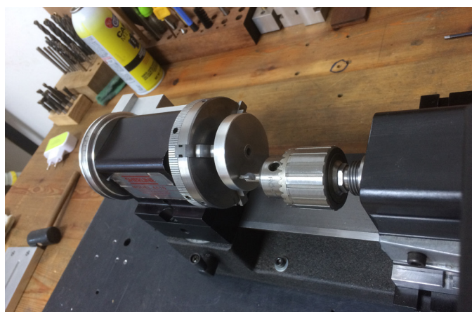
PICTURE 8—Another view of the headstock on the crossslide.
