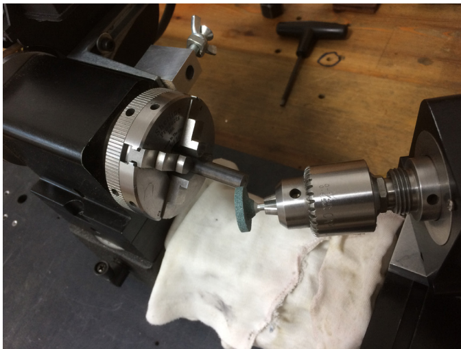
PICTURE 10—The crossslide headstock is mounted on an angle. The alignment key has been removed in this setup.
