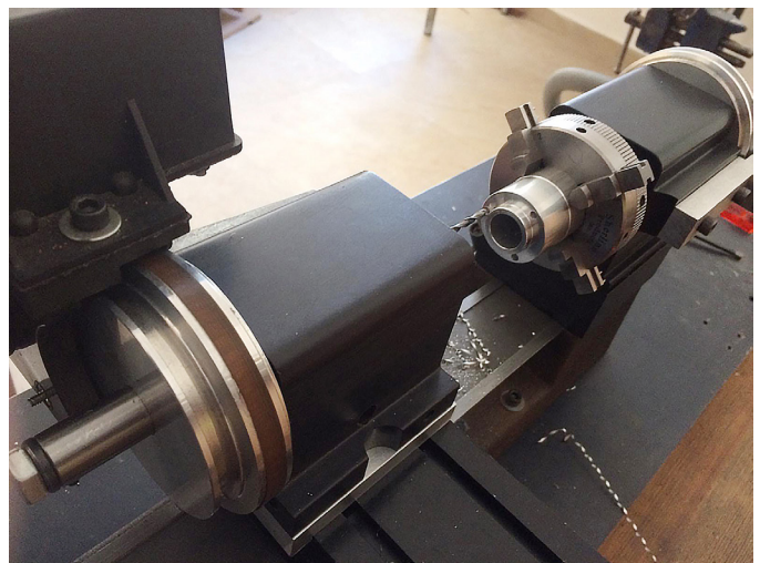
PICTURE 14— This application is doable on a lathe instead of using a rotary table and a right angle attachment on a milling machine.
