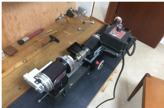
PICTURE 7—The motorized headstock mounted on the crossslide.
