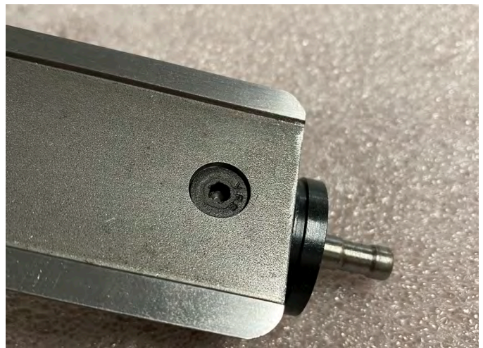
FIGURE 20—The 10-32 82° screw is now in place.
