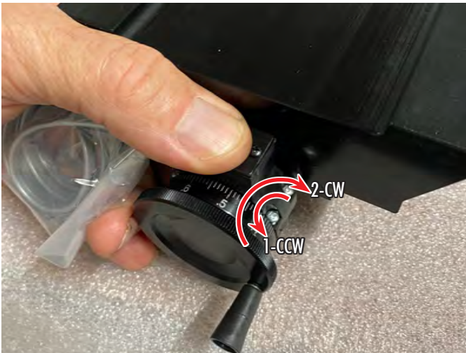
FIGURE 27—Note the numbers and the rotational arrows: 1: Rotate the screws CCW until the screw threads align with the existing housing threads. 2: Then tighten the screws CW until snug. DO NOT overtighten.
