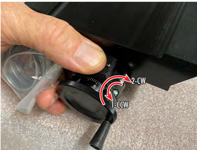
FIGURE 27—Note the numbers and the rotational arrows: 1: Rotate the screws CCW until the screw threads align with the existing housing threads. 2: Then tighten the screws CW until snug. DO NOT overtighten.
