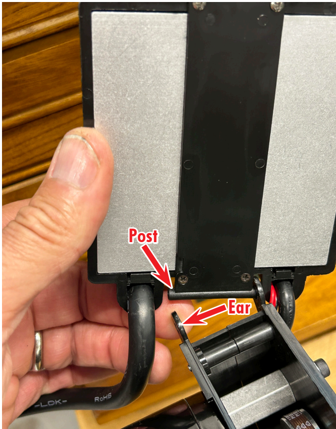
FIGURE 4—The posts are on the speed control housing and the ears are on the pulley belt guards.
