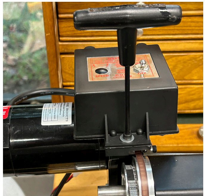
FIGURE 2—Use the 5/32" Hex T-driver to remove the locking screw from the housing.
