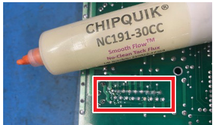
FIGURE 5—The red rectangle shows one of the four chip solder points.
