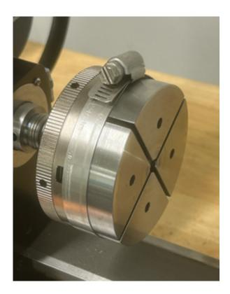
**Note:** Because of the clamp nut on the hose clamp, your chuck is no longer balanced and your machine will vibrate at higher rpms.
